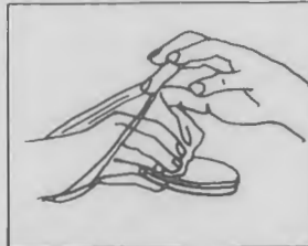
Peel bag over the hand turning it inside out while maintaining grip on biohazardous material.
